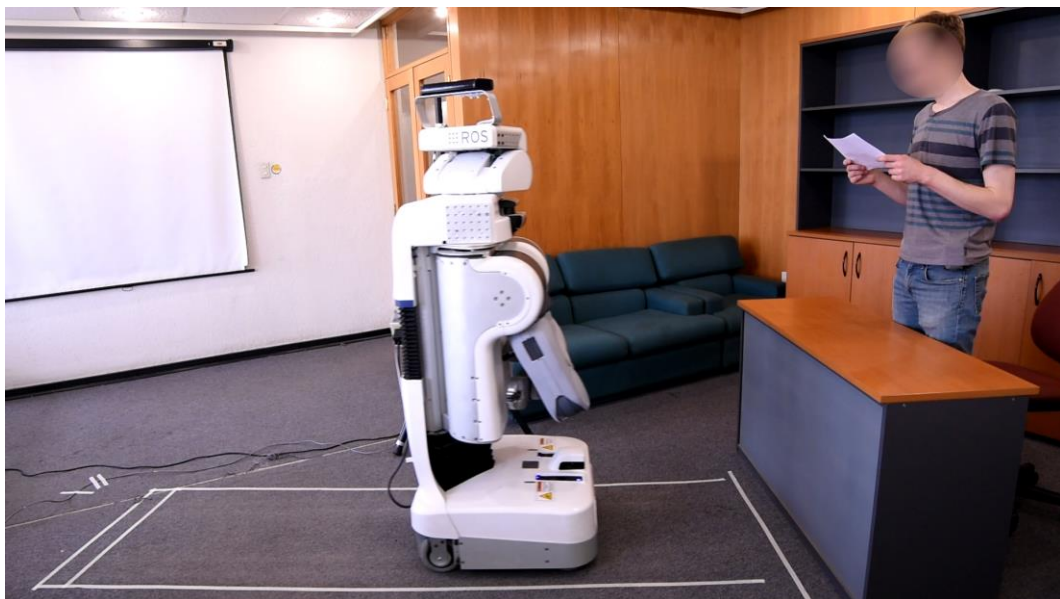
Figure 3.5 PR2 robot equipped with a Microsoft Kinect that was used to record the database: a) the source corresponds to a studio loudspeaker that was employed to reproduce clean utterances from a database; and, b) the source is a human speaker reading sentences from the same corpus.
