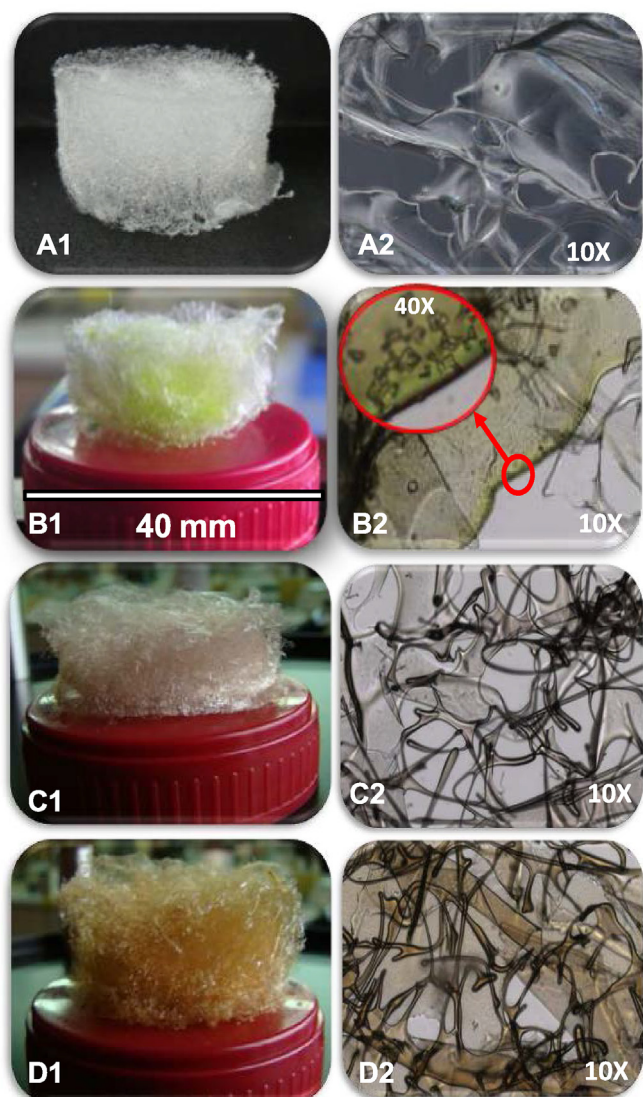
Fig. 7. Optical images without magnification ( \times 1 ) and magnified 10-fold ( \times 2 ) of aerogels made of CS/ChS (A1 and A2), CS/TPPS/ChS (B1 and B2), CS/TPPS/PV10/ChS (C1 and C2), and CS/TPPS/PK-Im/ChS (D1 and D2).
