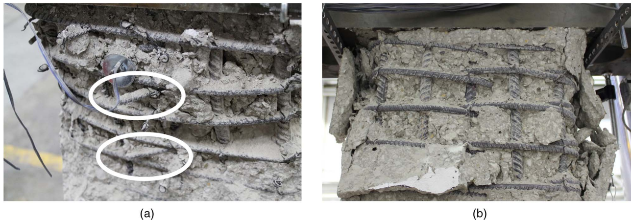
Fig. 10. Final damage state of a special boundary element: (a) with 90°–135° crossies (Specimen CS14); (b) with all rectangular hoops (Specimen CS1)
