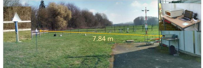
Figure 4: Picture illustrating the target measurement experiment. The prototype (on the right) emits a sinusoidal wave to the trihedral corner reflector (on the left) and registers the resulting echo power.
