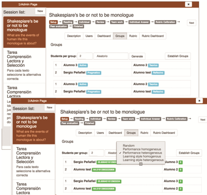
Fig. 3. Interfaces used by the teacher for the selection of the team members of a working group. The top view generated a random proposal; The bottom one is generated based on performance, with heterogeneous criterion: students with a good performance with others who did not perform well.
