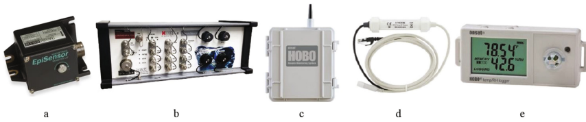
Fig. 1. Monitoring system installed in the church: (a) EpiSensor ES-U2 accelerometer sensor; (b) Obsidian 8x acquisition system; (c) HOBO RX-3000 Data Logger; (d) S-THB-M008 temperature/humidity sensor; and (e) UX100-011 HOBO environmental sensor.
