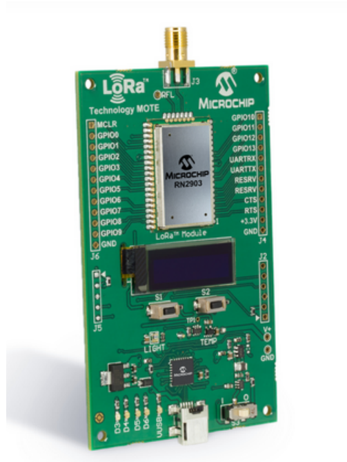
Figure 3.1: Microchip RN2903 LoRa Technology Mote, a device compliant with the LoRaWAN Specification version 1.0.2. It uses the [902 - 928] MHz ISM band.
