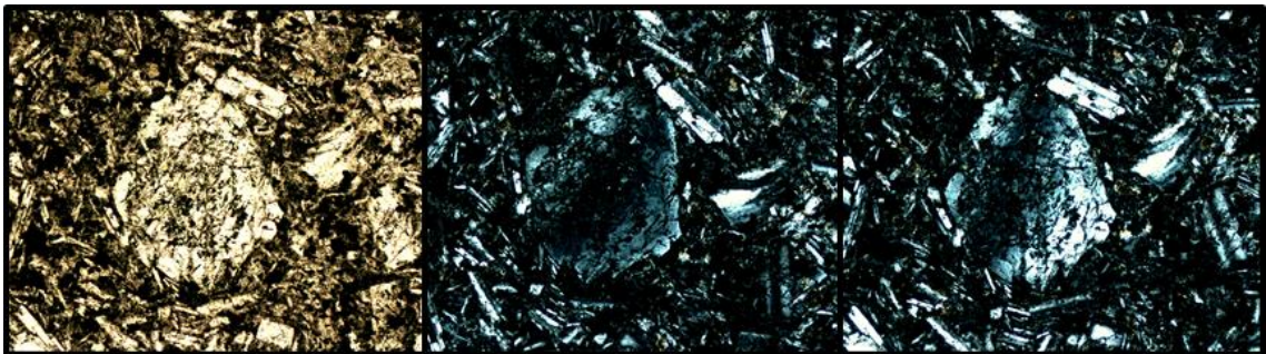
Figura 88: Unknown phase with undulatory extinction, in NP and two times in NX, respectively (showing extinction). Long size image= 2 mm.
