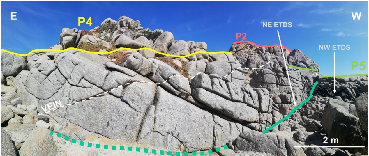
Figure 39. Panoramic southward view of P4 scarp (with inherent panoramic-effect distortion). Up: unedited panoramic field photo by author. Down: interpreted image showing an example of a NE-dipping fracture and vein (white dashed line). NW and NE ETDS are also shown. NE ETDS visible outcrop is indicated with a solid turquoise line, while the dashed line indicates its covered by in situ-formed sand. Photo-shot location and orientation shown in Annex 2.
