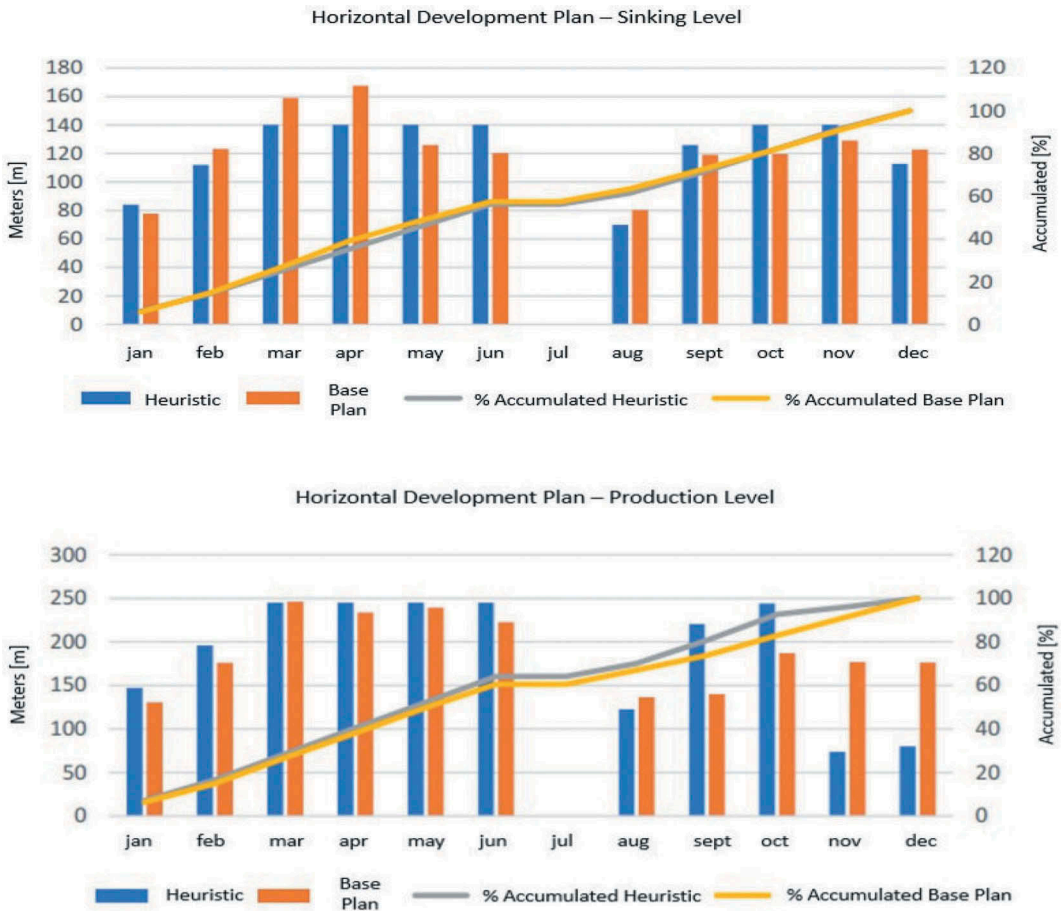
Figure 4. Horizontal development plan for undercut and production levels for the base development plan and the heuristic approach result.
