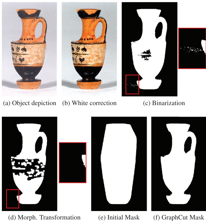
Fig. 4. The raw input (a) is subjected to histogram equalization (b) and thresholding (c). With morphological opening relicts of the background scenery are removed (d). The convex hull of all remaining connected components (e) is used for a graph-cut extraction (f).
