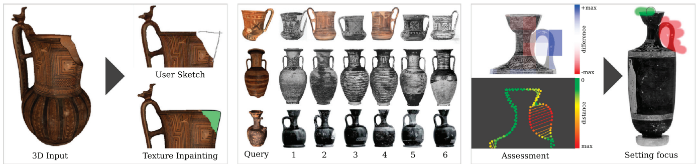
Fig. 1. Our proposed system. Left: The user specifies missing geometry of an incomplete 3D model by sketch and automatic texture filling. Middle: The retrieval returns similar objects in a ranked list. Right: Using dedicated visualizations, the results can be assessed and iteratively refined by setting foci.
