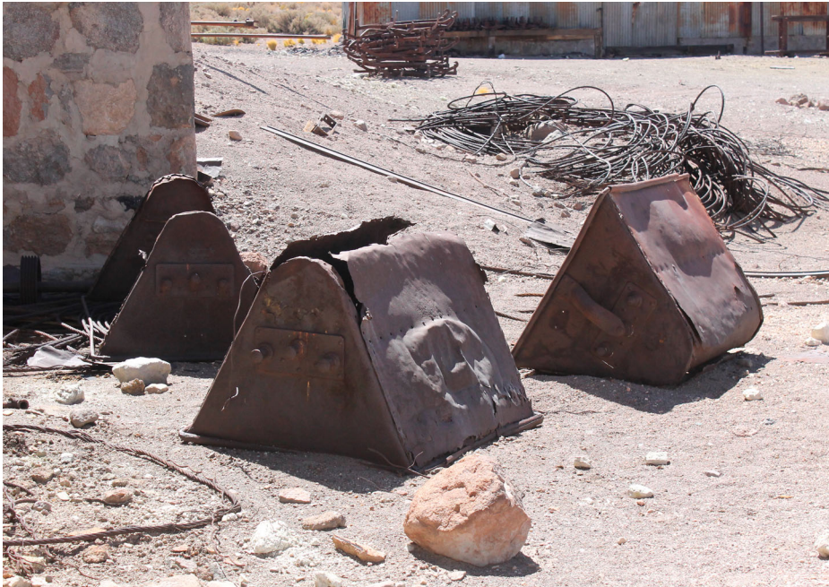
Figure 20. Aerial ropeway carriage remains on the Amincha discharge station. © Proyecto Arqueológico Alto Cielo.
