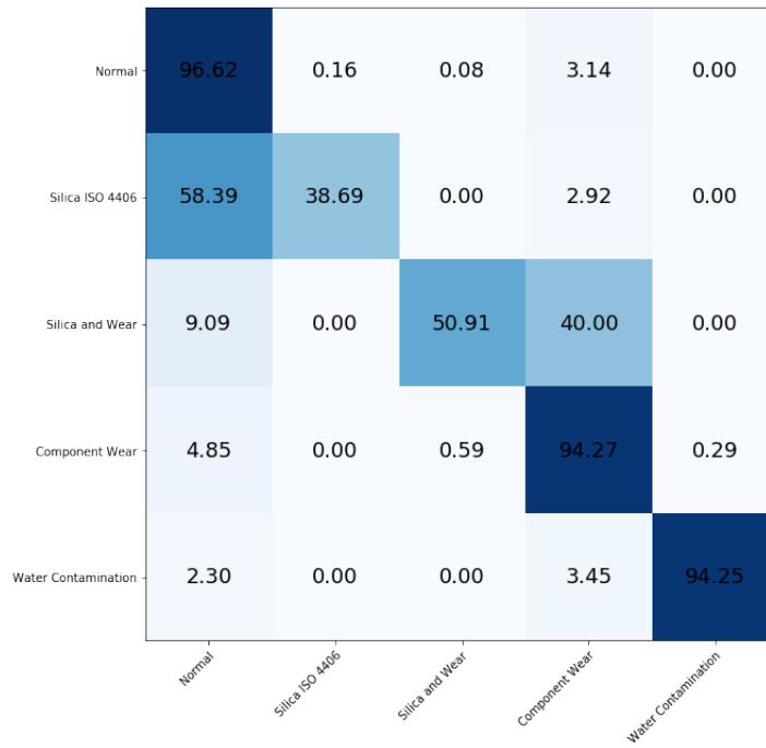
Figure 37: Flipout MLP - Confusion Matrix after-Filter
