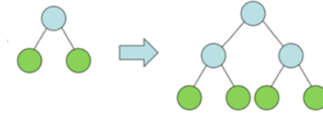
Figure 9: XGBoost Level-Wise Growth Mechanism
