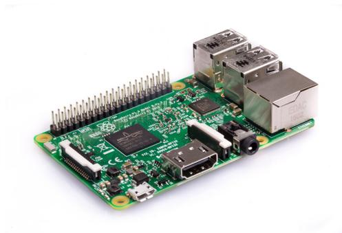
Figura 1.1: Raspberry Pi 3 Modelo B
