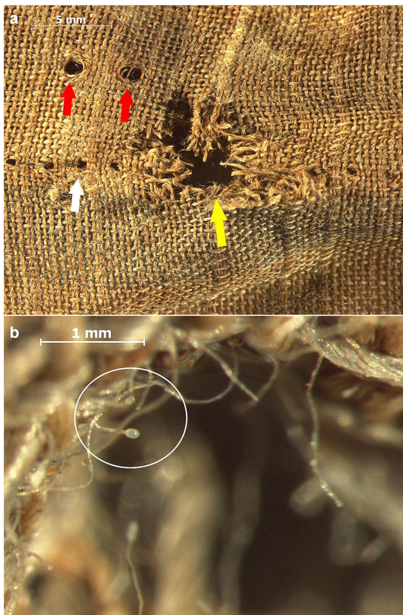
Figs. 5-7 a–c A bullet hole in a synthetic shirt (white arrow: seam; red arrows: button's holes; yellow arrow: bullet hole) with globular fibre ends in the margin (white circle) (case no. 5)
