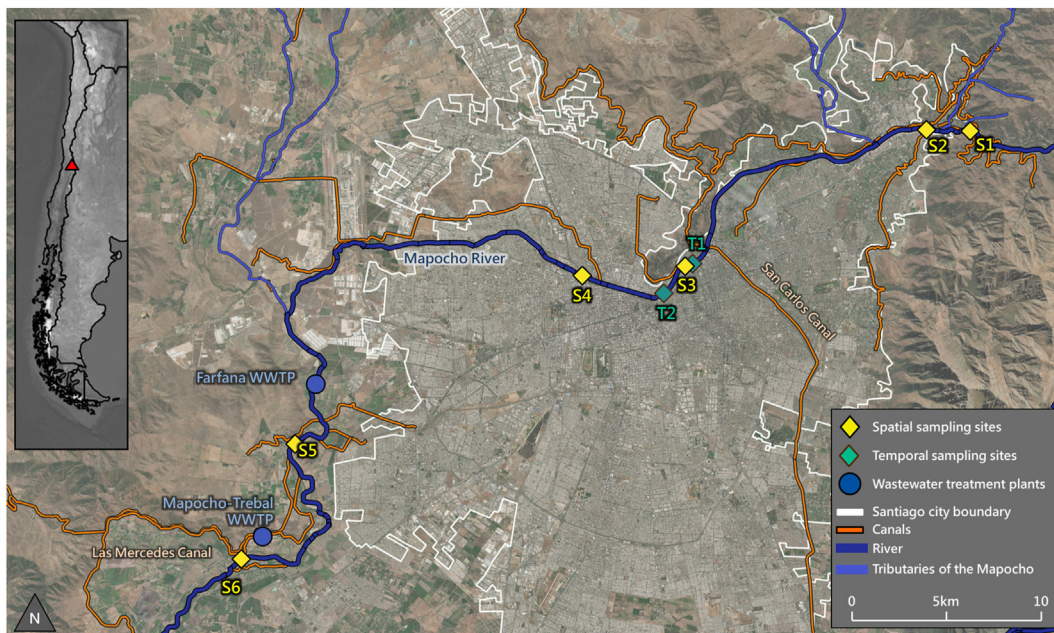
Fig. 1. Map of sampling locations. S1 to S6 are spatial campaign sampling locations. T1 and T2 are temporal campaign sampling locations. Both wastewater treatment plants (WWTP) discharge into the Mapocho. The San Carlos Canal discharges a variable portion of its flow to the Mapocho; all other canals indicated extract water from the Mapocho. River geometry is from Digital Chart of the World (Digital Chart of the World, n.d.). Channel geometry is from the Chilean Ministry of Agriculture (Chilean Ministry of Agriculture, n.d.). City boundary geometry is from the Chilean Ministry of National Goods (Chilean Ministry of National Goods, n.d.). The basemap is used courtesy of ESRI.
