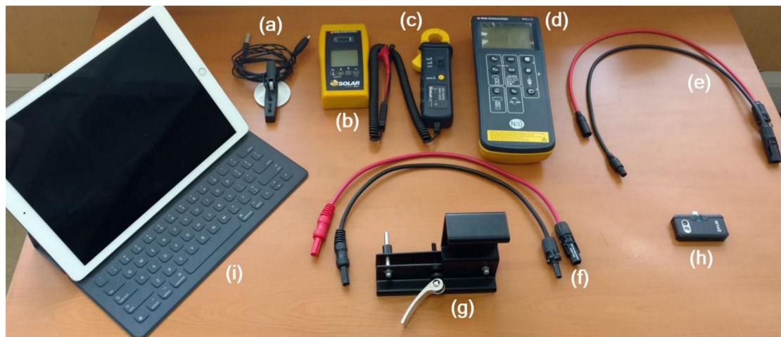
Figure 2. Minimum equipment and tools for data collection in the field. (a) Temperature sensors. (b) Irradiance sensors. (c) Direct current (DC clamp) ampere-meter. (d) Current-Voltage (IV) tracer. (e) MC3 to MC4 adapter leads. (f) MC4 tests leads. (g) Irradiance meter mounting bracket. (h) FLIR ONE pro camera. (i) iPad.
