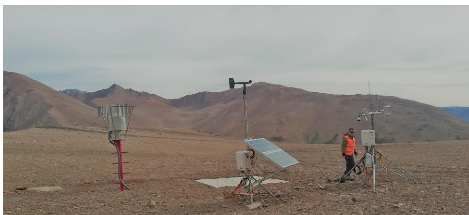
Figure 2. La Ollita meteorological station and the snow scale, on 15 December, 2015 (photo by Miguel Lagos).
