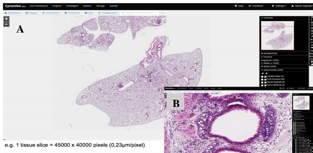
Fig. 1.4. Example of the Cytomine interface for the visualization of WSIs. Cytomine is an open source slide viewer. Two separate windows can be observed in this figure. Window A shows the WSIs with the maximum zoom out. Window B shows a zoom in on a specific region. Both windows present a menu on the right side, containing a map of the WSI and buttons to toggle annotations. Source: [30]
