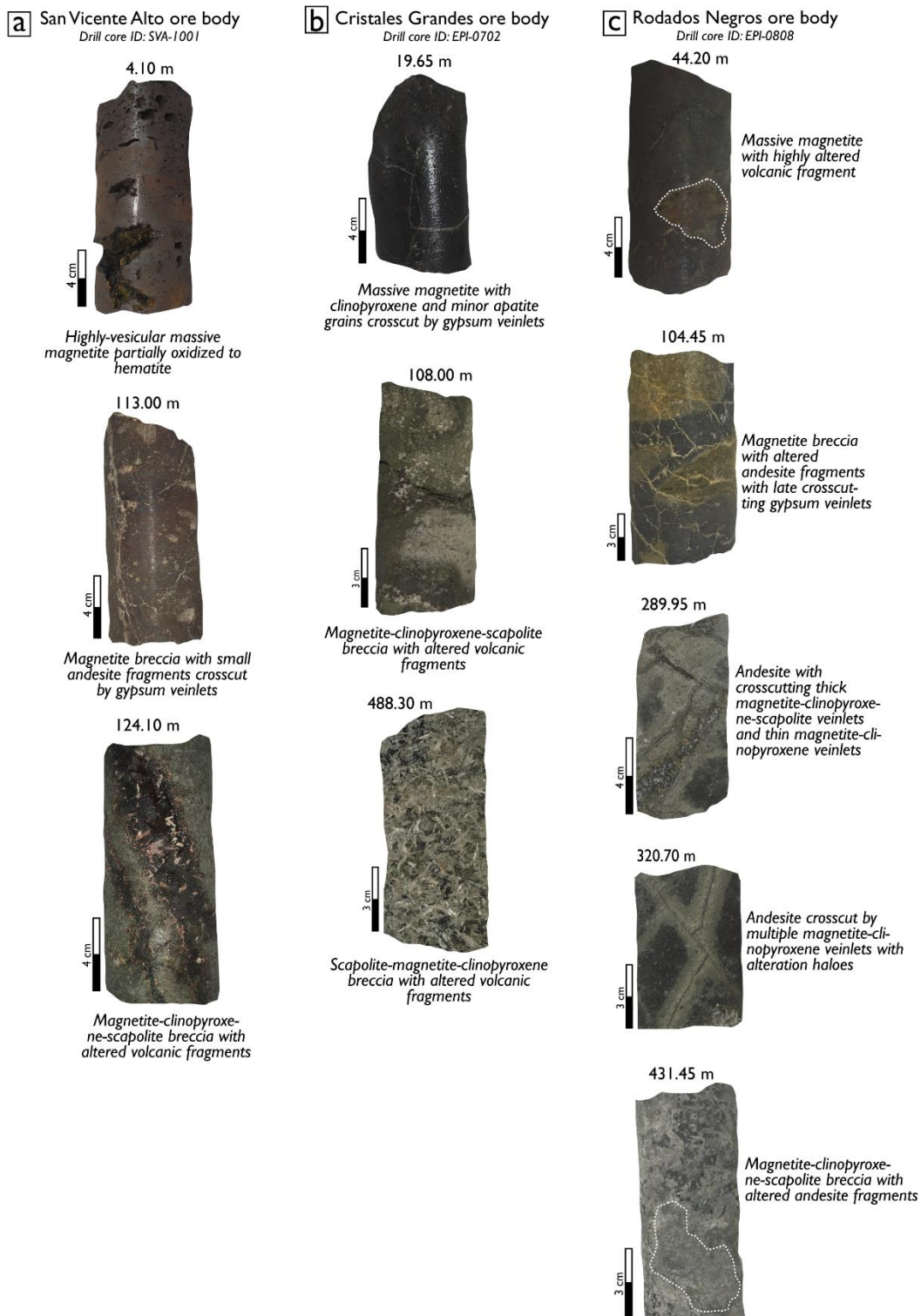
Supplementary Figure B2: Photographs of the drill core samples from the El Laco magnetite ore bodies. (a) SVA-1001 drill core from San Vicente Alto ore body. (b) EPI-0702 drill core from Cristales Grandes ore body. (c) EPI-0808 drill core from Rodados Negros ore body. Photographs display the transition from massive magnetite at surface/shallow depths to magnetite breccias at depth; some host veinlets.
