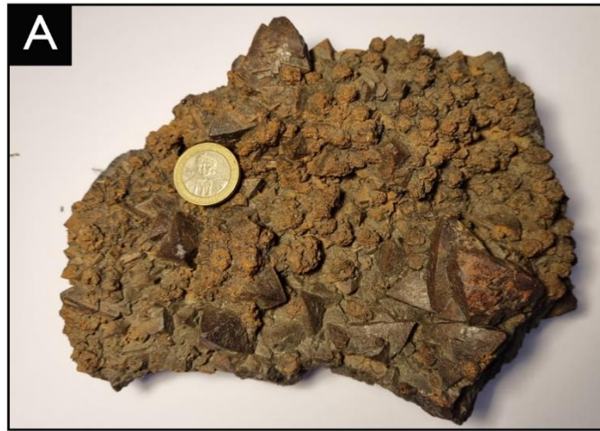
Supplementary Figure C3: (A-C) Hand-sample ore specimen from Laco Norte ore body showing centimetre-scale well-developed octahedral magnetite associated with abundant spherical structures formed by magnetite.
