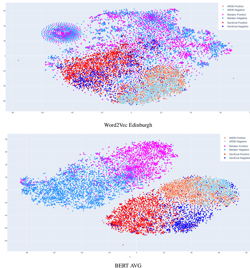
Fig. 5: 2D visualization of all sentiment training datasets projected to the same space using t-SNE for both BERT AVG and Word2Vec Edinburgh representations. Point colors indicate the sentiment/dataset combination associated with each example.
