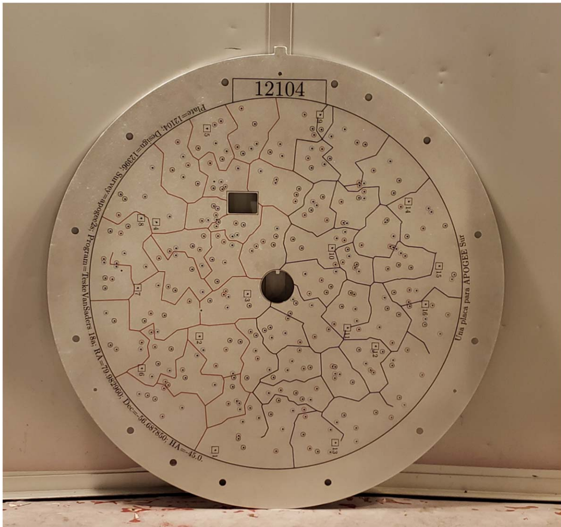
Figure 1. Example of an APOGEE-2S plate. APOGEE-S plates cover a smaller area on the sky than APOGEE-N plates (due to telescope plate scale differences), and they also have a slightly different layout (compare to Figure 13 in Majewski et al. 2017). Most obviously, there is a central hole for an on-axis acquisition camera and another rectangular hole for an off-axis camera. These fiber exclusion regions are taken into account in the target selection and plate design software. Another difference with APOGEE-N plates is that all plate markings, including coding of the holes to denote bright, medium, and faint fibers, are automatically printed for the APOGEE-S plates, whereas they are hand-marked for the APOGEE-N plates (the coding may not be visible without enlarging the image). Photo by R. Beaton.
