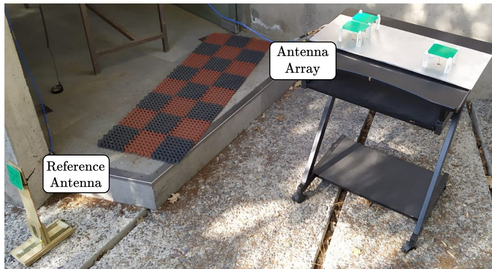
Figure 6.8: Antennas configuration to take measurements.
