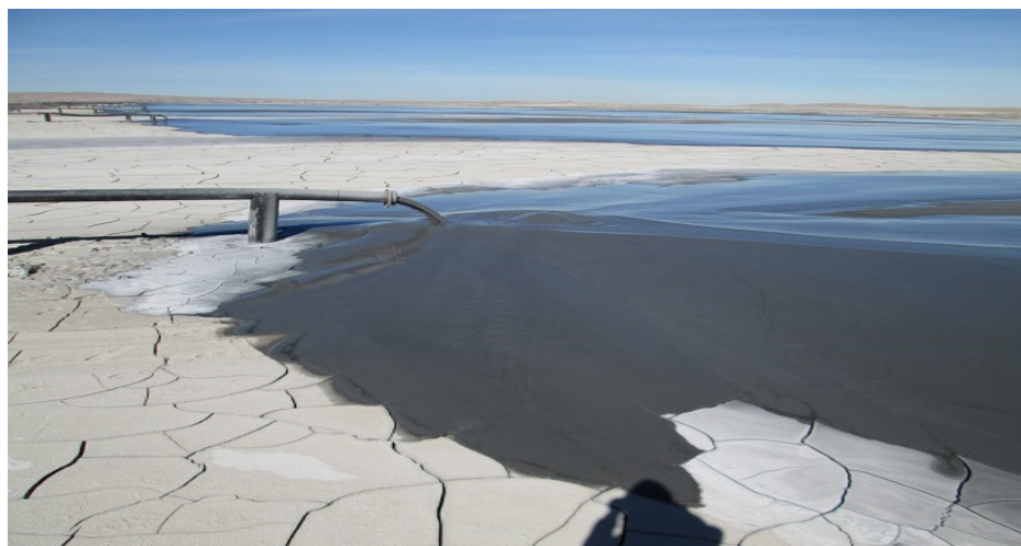
Figure 7. Thickened Tailings Technology—Esperanza TSF Centinela Mine Chile [11].
