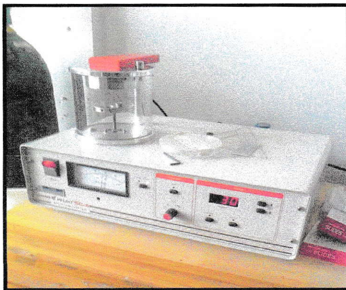
Figura 11: Sputter Coater Pelco SC-6.
