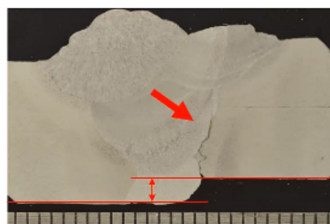
Figure 1.1: Cracking due to misalignmen
