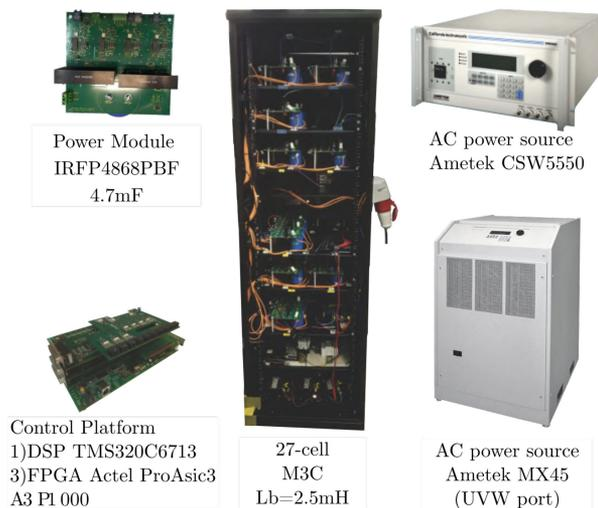
Fig. 9. Experimental setup of an  $M^3C$ .
