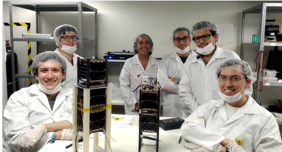
Figure 1. Images of the SUCHAI-2 and -3 CubeSats during the integration process together with part of the development team at the Space and Planetary Exploration Laboratory (SPEL). The launch of these CubeSats is scheduled for 2022. They will carry magnetometers and a communication system to receive the data from two femto-satellites. Each of these femto-satellites will also carry a magnetometer. The femto-satellites will be carried and deployed by the SUCHAI-3 CubeSat. We are studying the feasibility of estimating the location of a radio source (femto-satellite) in a concrete scenario, in low earth orbit where there are only two CubeSats available to estimate the location of two femto-satellites in a future mission.
