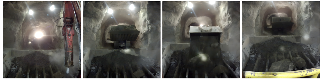
Figure 1. Interaction between an LHD dumping material onto the grizzly, and a hydraulic impact hammer. When the LHD is approaching the grizzly, the impact hammer moves to a safe position.
