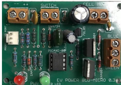
Figura B.3: Battery Management System EV POWER BCU-MICRO 03.
