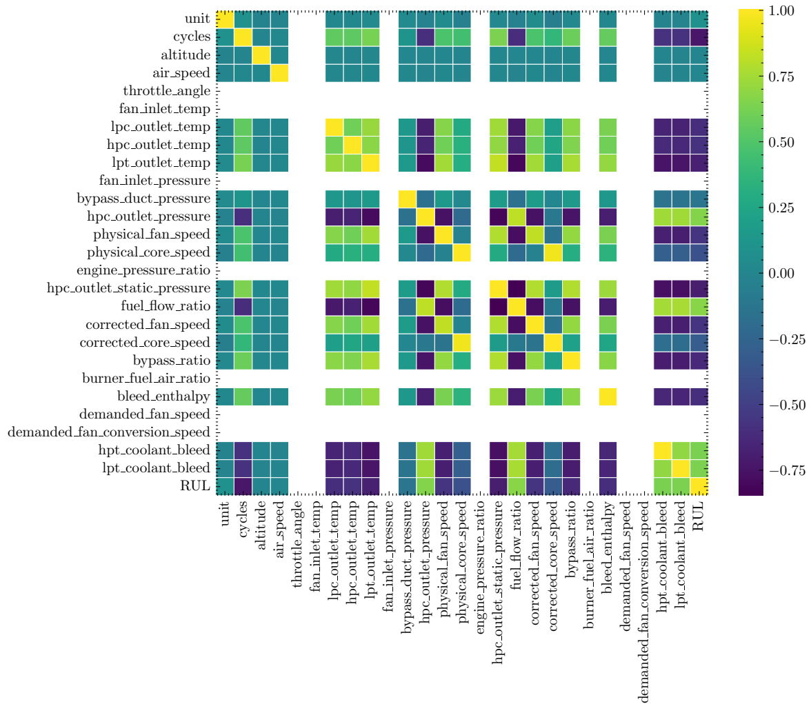
Figure 4.1.5: C-MAPSS Aircraft Correlation Matrix Between Features
