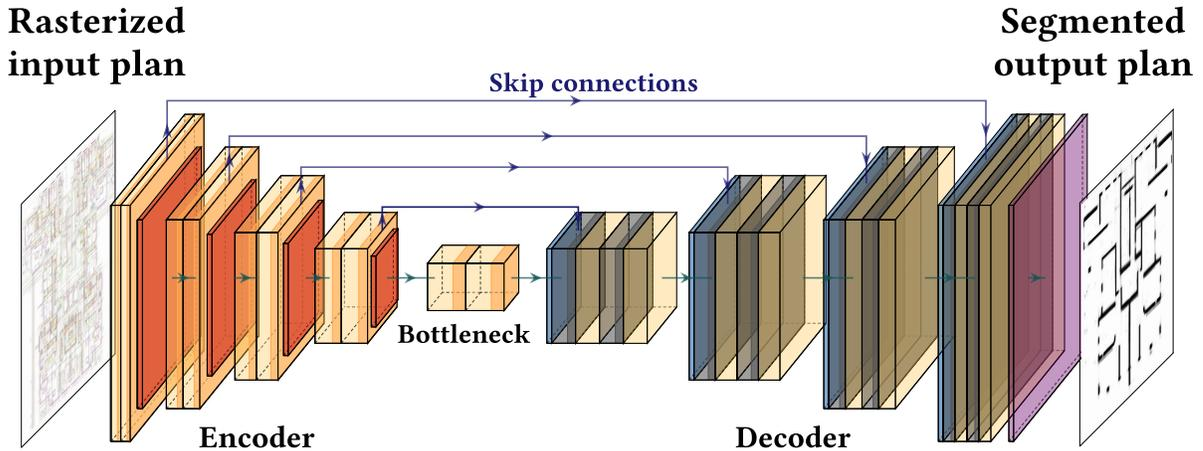
Figure 2.9: A U-Net model which segments the walls from a rasterized floor plan image. Layer legend: (yellow) convolutional block, (orange) max-pool, (blue) up-sampling, and (purple) softmax.
