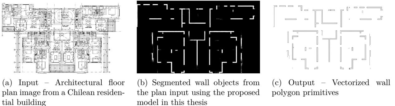
Figure 1.1: Inputs and outputs of the proposed model.
