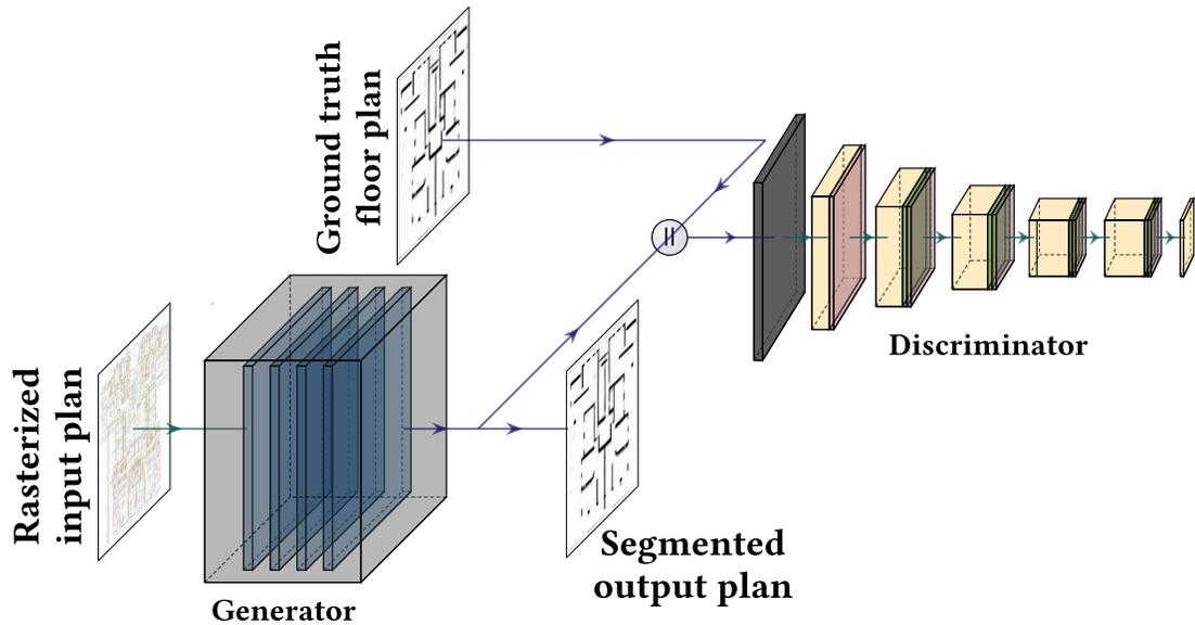
Figure 2.11: Pix2Pix model that translates the rasterized floor plan image style into a segmented format.
