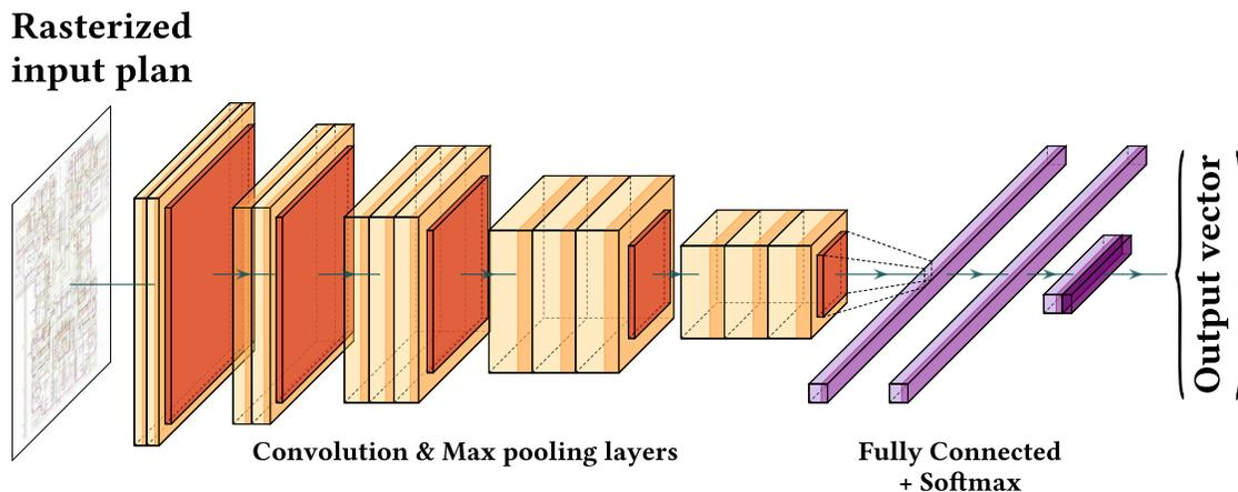
Figure 2.5: VGG model architecture, which extracts features from a rasterized floor plan and outputs a vector that can be used to predict or classify several elements.
