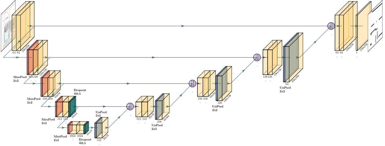
Figure 3.6: U-Net model architecture implementation, which takes each floor plan crop patch as input, and returns the segmented plan as output. Layer legend: (yellow) convolutional block, (orange) max-pool, (blue) up-sampling, and (green) dropout.
