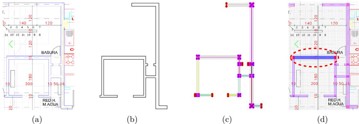
Figure 3.2: Example of the MLSTRUCT-FP’ wall assembly process – (a) retrieval of the floor plan image, (b) wall contour polygon retrieval from its CAD model, (c) wall polygon disassembly into a rectangular segments graph, (d) modeling of the wall, where a rectangle is highlighted [21].
