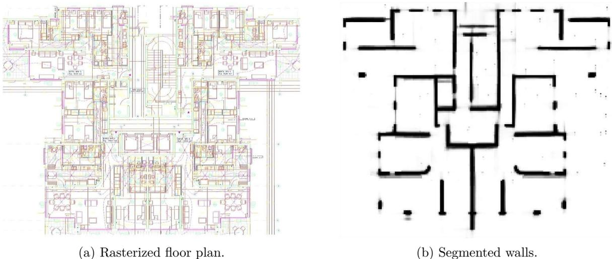
Figure 2.6: Example of segmented walls from a floor plan image.
