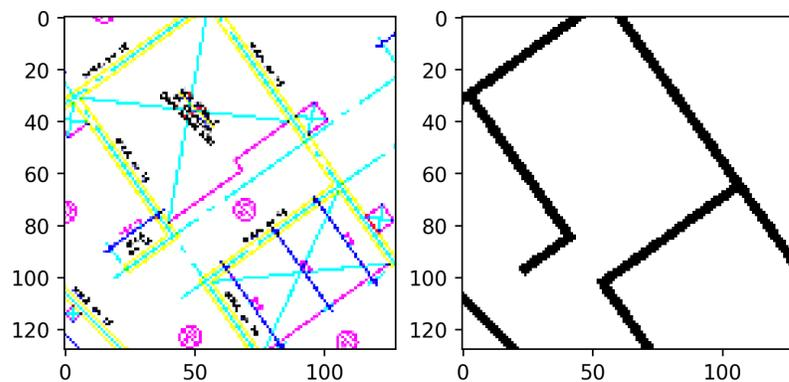
(b)  $128 \times 128$  px crop of a  $7.5 \times 7.5$  m region with a  $45^\circ$  clockwise angle rotation. Factor 0.058 m/px
