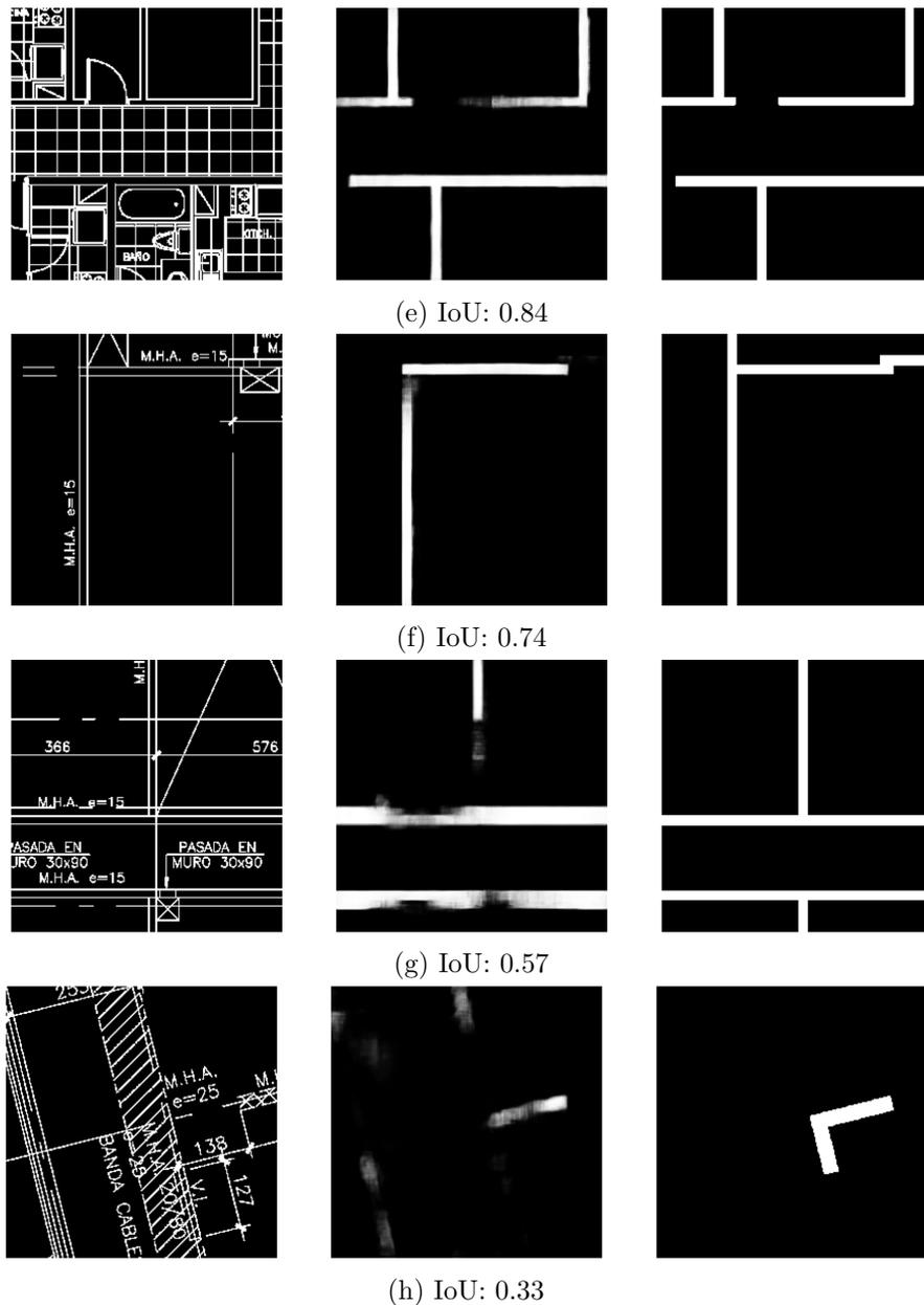
Figure 3.9: U-Net model results for different patches considering a  $256 \times 256$  px image and  $5 \times 5$  m crop area. Each image displays the input (patch crop), the model result (segmented wall), and the ground truth (continuation).
