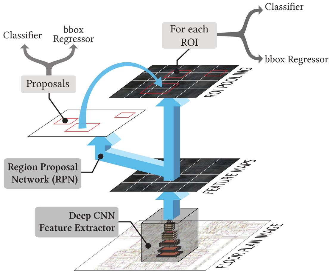
Figure 2.10: Instance segmentation Faster R-CNN model [69] that considers a floor plan image as input and predicts the position of the objects inside region proposals.
