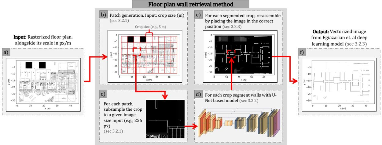
Figure 3.4: Schematic of the wall retrieval method from rasterized floor plans proposed in this thesis.
