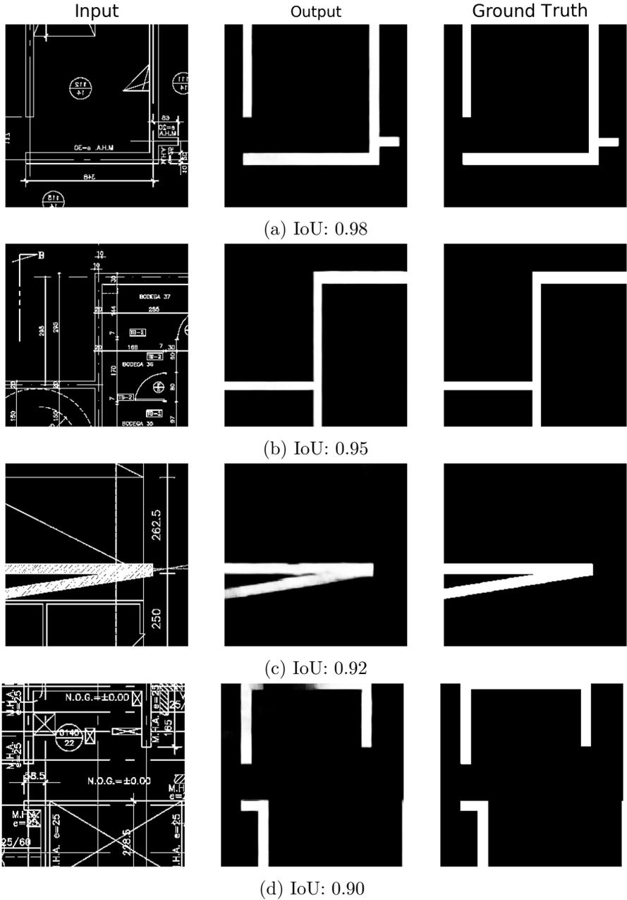
Figure 3.9: U-Net model results for different patches considering a  $256 \times 256$  px image and  $5 \times 5$  m crop area. Each image displays the input (patch crop), the model result (segmented wall), and the ground truth.
