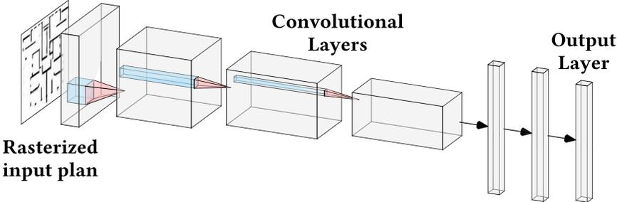
Figure 2.7: Generic CNN-based model that automatically retrieves features from a rasterized plan, for example, to segment walls or classify its objects.
