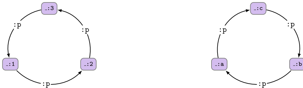
Figure 3.4: Two isomorphic RDF graphs. The bijection M is M(1) := a , M(2) := b , and M(3) := c .
