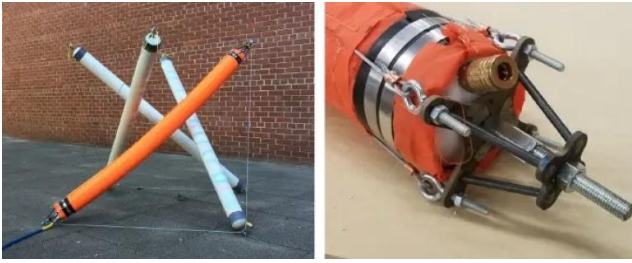
Fig. 8: Prototipo y detalle de control de aire. Fuente: Deployable Tensegrity Structures with Inflatable Compression Struts.
