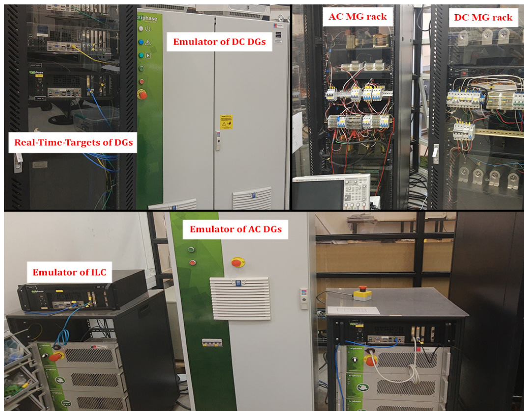
Figure 3.8: Components of experimental testbed hybrid AC/DC MG, described in [3]. Reproduced from [2].
