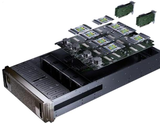
Figura 38: Supercomputadora DGX-1 (<https://www.amax.com/wp-content/uploads/2020/01/DGX-1-IMG.png>).
