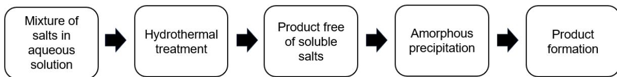
Figure 3-4: Involved process in the production of laponite (Pardo Ojeda, 2020).
