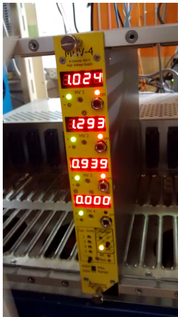
(a) High voltage unit model MHV-4 Mesytec, used in WAS3ABi.
