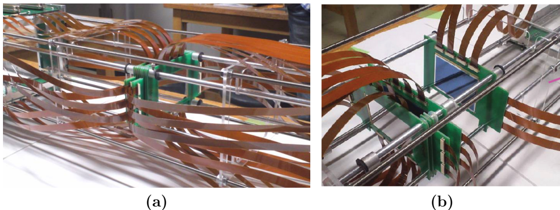
Figure 3.1: Picture of WAS3ABi DSSSDs without the aluminum cover. Each side of the DSSSD, the X and Y sides, is composed of strips. The end of each strip is connected to a HUB that it was connected to the pre-amplifier.
