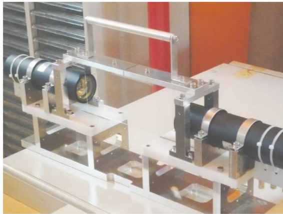
Figure 2.7: Plastic scintillator picture from [Tea19]. Each plastic detector used in BigRIPS has two photomultipliers attached on the edges.
