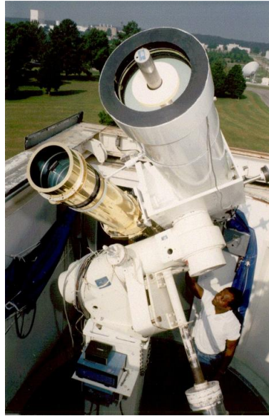
Figure 2.1: Photograph of MSFC (Marshall Space Flight Center) magnetograph. James Smith (retired), former chief observer, is shown besides the instrument. Photograph taken from NASA repository https://magnetograph.msfc.nasa.gov
