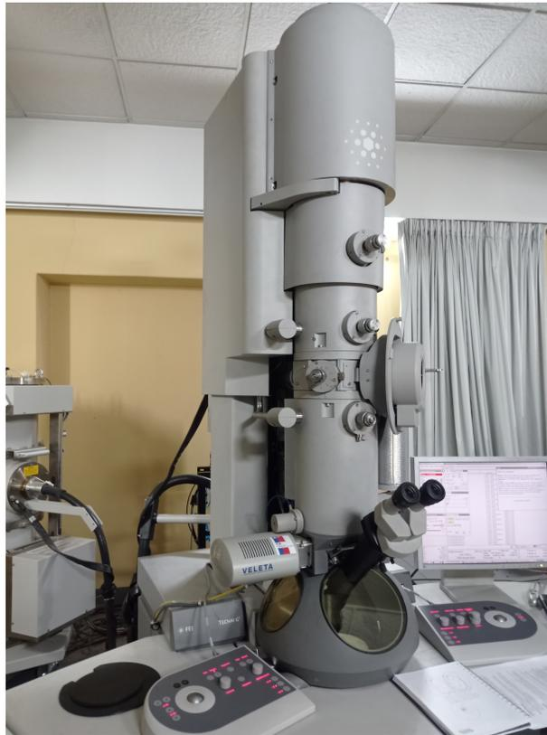
Figura 3.7: Microscopio TEM FEI Tecnai G2 F20 S-TWIN 2005
